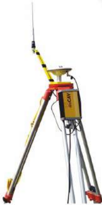
GPS BASE STATION
