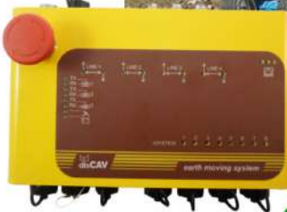
GNSS RTK RECEIVER & HYDRAULIC CONTROL BOX
